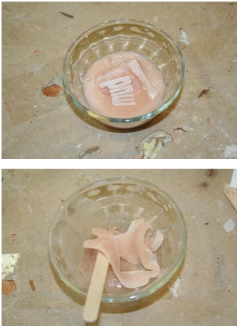
Shown counterclockwise from top left: Melting gelatin; gelatin flashing (to reuse); mold halves and gelatin cube.
