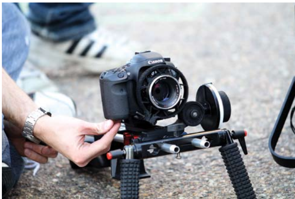
The Canon 7D with a Nikon lens adapter and cinema setup on the set of Breakaway . Photo courtesy of Jason Anderson.
